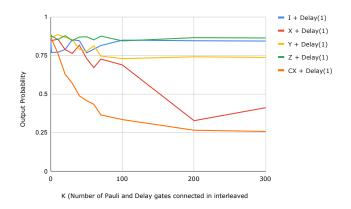
Fig. 5. K vs. Output Probability plot where malicious circuit is Pauli gates and delay gates connected in interleaved fashion; data for CNOT gate experiments is shown for comparison.
