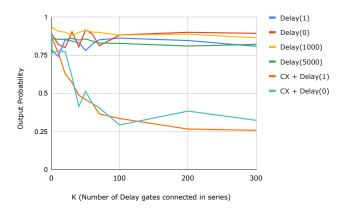
Fig. 4. K vs. Output Probability plot where malicious circuit is series of delay gates, delay length in units of dt is given in the parenthesis in the legend; data for CNOT gate experiments is shown for comparison.
