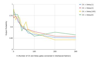
Fig. 3. K vs. Output Probability plot where malicious circuit is CNOT (labled CX in the figure) and delay gates connected in an interleaved fashion.
